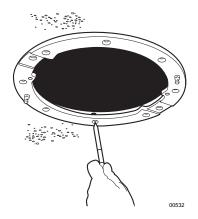
c. Use the mounting ring as a template and mark the hole pattern onto the mounting surface. Prepare the holes.
